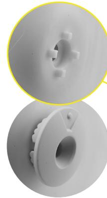
Ensure the canting is positioned correctly before tightening. The canting must be flush with the shell.
